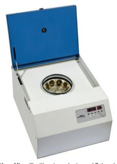
Centrifuge Micro III with universal rotor and Babcock sleeves
